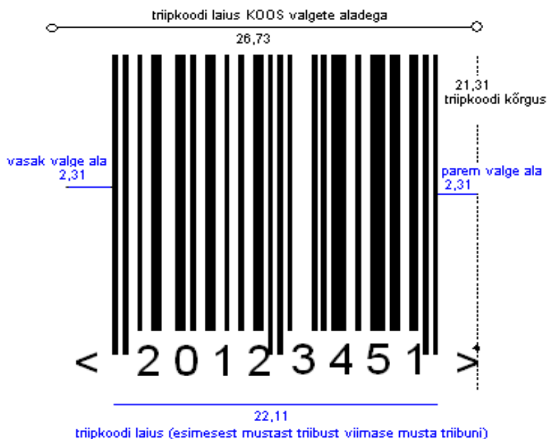
Figure 24 - EAN8, 100% scale ratio (millimetres)
