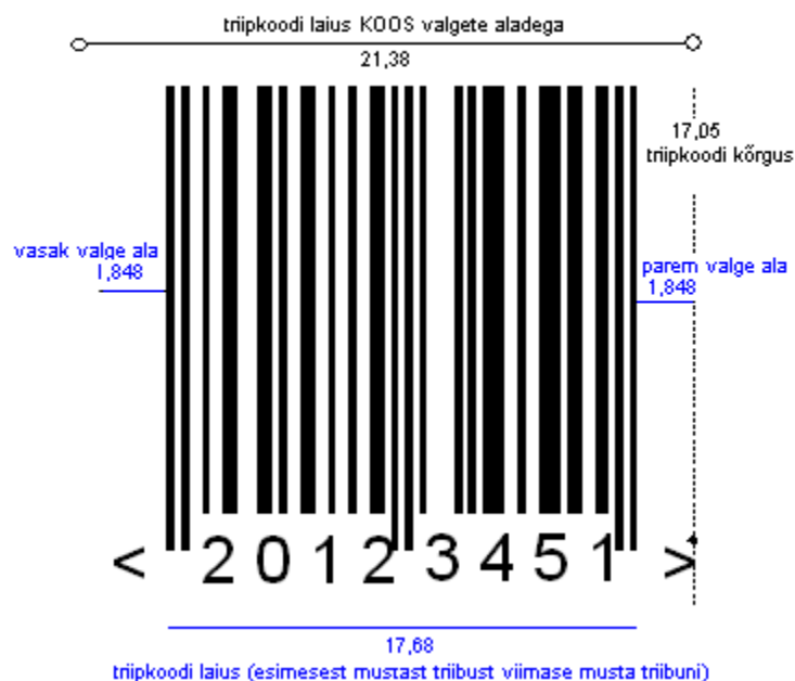
Figure 23 - EAN8, 80% scale ratio (millimetres)
